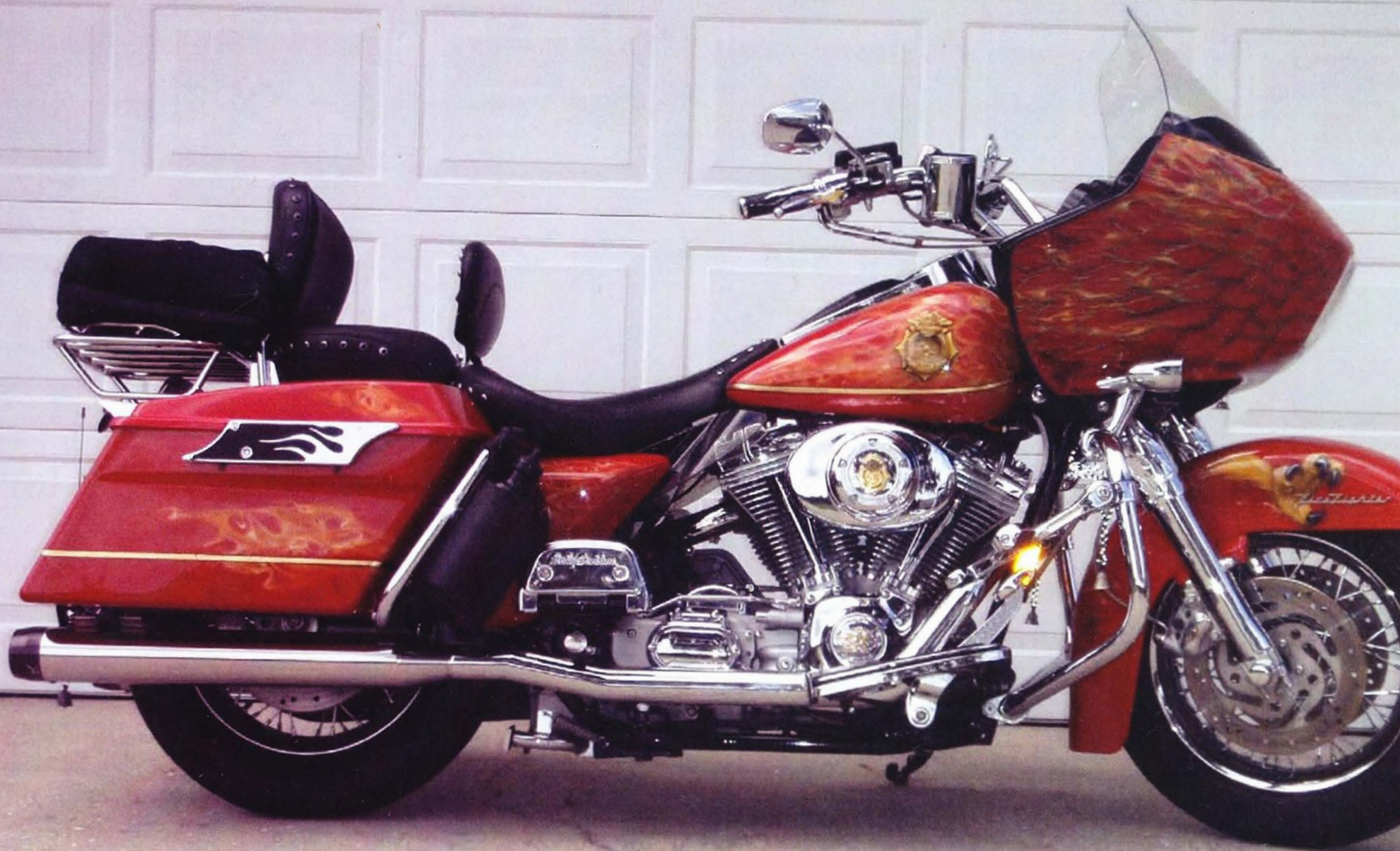
Two Up – Folding Back Rest for Driver, Fixed Backrest for Rider Detachable Two Up Luggage Rack with Removable Luggage Bag
